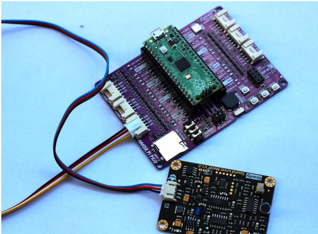
Because **Sound Level Meter** sensor is **analog**, then we must connect them to GP26, GP27 or GP28- analog ports of Raspberry Pi Pico. In our case the best way is select GP27 or GP26 (we have grove socket on the shield Maker Pico connected to these pins). Below
