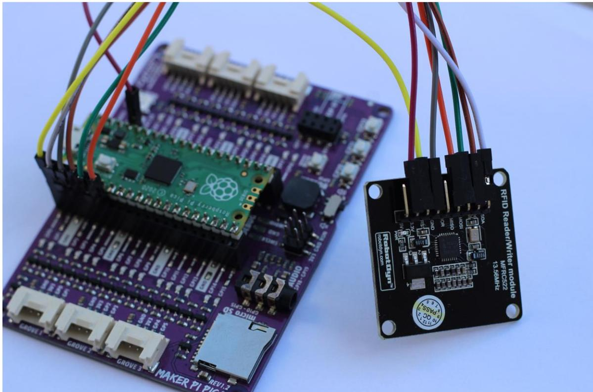
RFID reader use serial communication in **SPI standard**, so we need a bit more wires then in I2C case.
